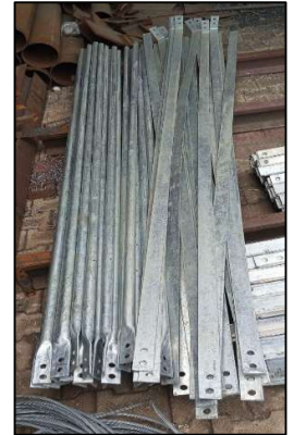
Pipe Type Earthing
